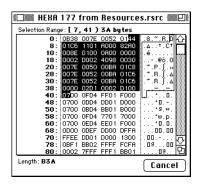
Below the lower left corner of the scrollable area, the Editor shows you the current length of the data, measured in bytes. Initially the value is displayed in hex, but will be in decimal if you have chosen **Decimal Offsets** in the **Hex** menu.
