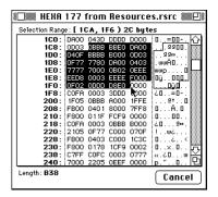
data. The values of the start and end of the range are constantly updated in the upper left corner of the window, so that you can make accurate selections in the middle of lines.
