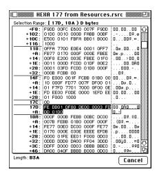
When this mode is in effect, the first byte of every paragraph continues to be displayed relative to the start of the resource, since it would otherwise always be 0 (an elegant but altogether useless piece of information). Subsequent lines in the paragraph have offsets that are preceded by a plus sign '+' to indicate that they are relative to the offset of the beginning of the paragraph.
